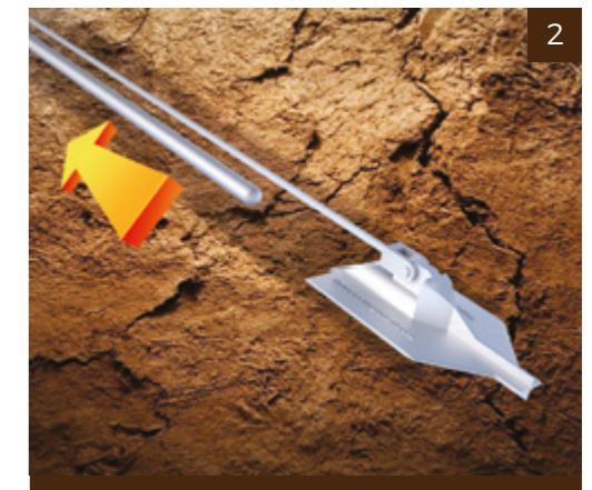
Pulling out the steel drive perch
